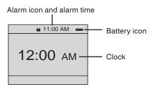
Press **STANDBY** again to return the IS9181 to standby mode. When in standby mode, the IS9181 exits menus, stops the music, and the backlight on the VTech logo turns off. The clock appears while in standby mode.
